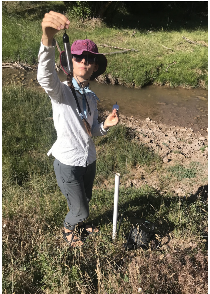
Holding up a pressure transducer, used to measure groundwater level
