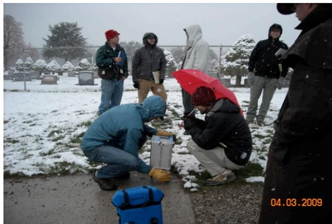
Students set up a gravimeter to measure the proposed Pechman Tear Fault.
