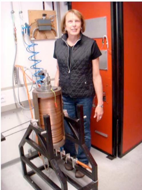
*Barb Nash stands next to the internally-heated high-pressure autoclave at Leibniz University in Hannover, Germany, that she used for her melting experiments on rhyolite erupted from supervolcanoes of the Yellowstone hotspot.*
