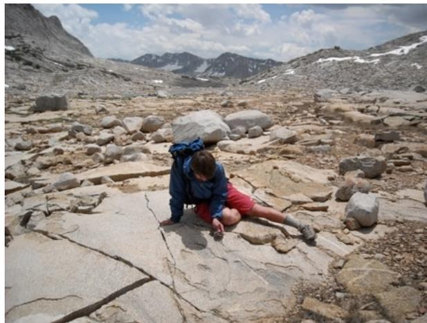
*Mike Stearns (M.S., 2009) measures the orientation of an offset across a minor fault related to the West Pinnacle fault zone in the Sierra Nevada, California.*
